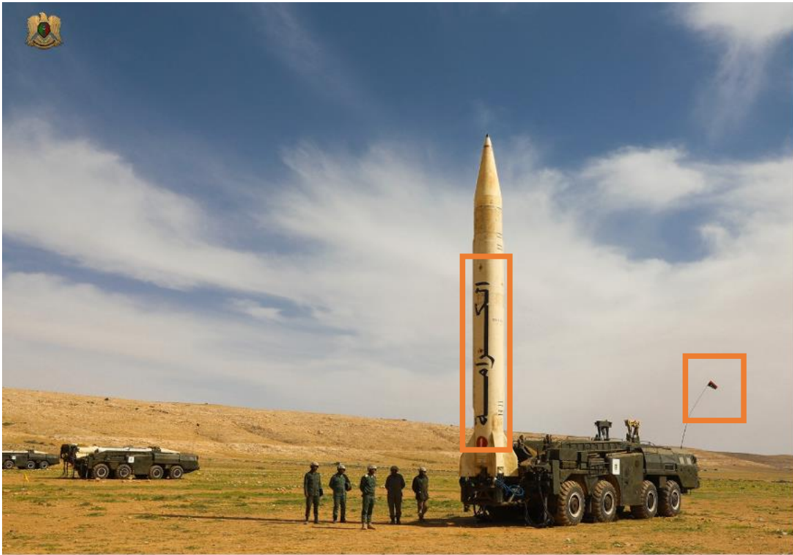
Figure 103.7 TBM on TEL in launch position
